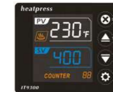
Clear Counter NO. You can long hold the CLEAR button to clear the COUNTER NO. on the panel.
