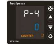
P-4 : Auto Power-off Mode Touch SET & ↑↓ buttons to set auto-off time with 0-120 mins range
