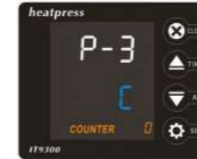
P-3 : °C or °F Read-out Touch SET & ↑↓ buttons to set °C or °F
